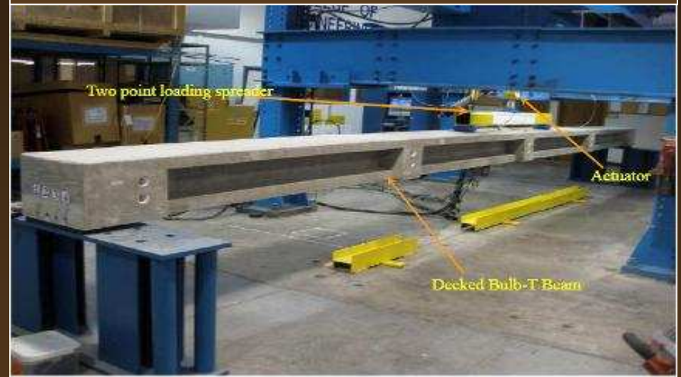
Ultimate Load Test Setup of Control Beam
